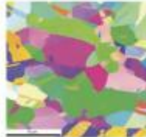
EBSD image (OIM) made on an as-cut surface of copper
